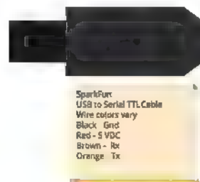
Figure 2. Prototype hardware using a USB to 3.3 VDC TTL serial cable. Includes an LED for the Teleduino demo.
